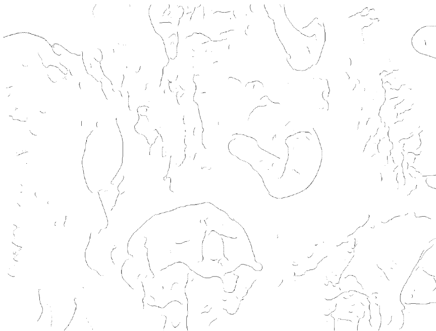
Figure 15. Multiscale edges calculated from the pseudo-gravity transform of Fig. 13 at scale s = 5 ( z = 5z_0 ).
