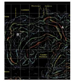
"Worms" at coarse scale: A = edge of Carbonate province, B = embayment through Salt Deformation Province; possibly relative to a deeper structure.
