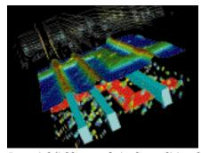
Potential field anomaly in the traditional form, (middle), 3D corresponding sheets (top). Demonstrative estimation of the shape and depth of the causative source (bottom). A potential field anomaly is represented in the traditional form, and, on top of it, the set of 3D corresponding sheets. Analysis of each anomaly can be performed individually by clicking on the corresponding sheet.
