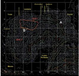
"Worms" at fine scale: A = edge of carbonate province, B = edge of Sigbee Escarpment, and Zone 1 = Self Deformation Province with different "worm" texture to Zone 2 (Hemipelagic deposits).
